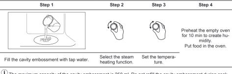
(1) The maximum capacity of the cavity embossment is 250 ml. Do not refill the cavity embossment during cooking or when the oven is hot.
