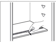
To remove the humidity control device, open the drawer below the glass shelf and pull out the cover.
