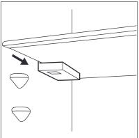
**Replacing the CleanAir+ filter** 1. Open the plastic housing.
