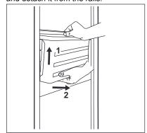
Push the rails inside the cabinet to avoid damage to the appliance when closing the door.
