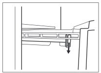
3. Pull the drawer out while lifting it up and detach it from the rails.
